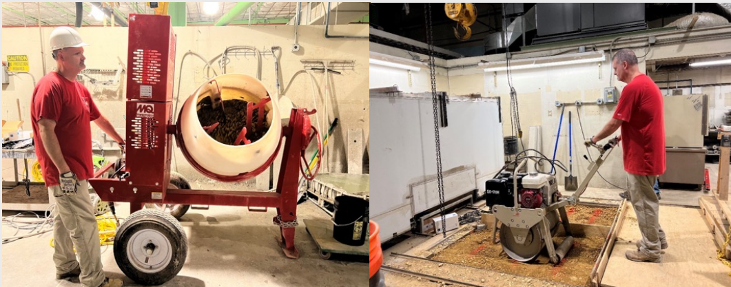
Uniform mixing and vibratory compaction in the pit
